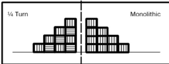
The diagram shows quarter turn and monolithic installation methods: For the monolithic method all backing arrows should point in the same direction. For the quarter turned method the backing arrows should be at a ninety degree angle to each other with all vertical arrows pointing in the same direction and all horizontal arrows pointing in the same direction at a ninety degree angle to the vertical arrows.
