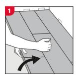
Separate the entire row by carefully lifting up at an angle. Fold up the row and release the whole long side.
