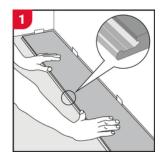
First row, first plank Starting from the left-hand corner, place %" spacers against walls on each side and place the first plank with the groove side facing out.
