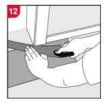
Trimming door and baseboard molding Position a plank with the decorative side down next to the existing door trim or baseboard molding. Using the height of the plank as a guide, cut to size using a hand saw as shown above.
