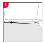
Starting the next row Place %" spacer against the wall and use either the cut part from the last row, or a new plank measuring at least 15" in length.
