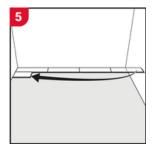
Starting the next row Place %" spacer against the wall and use either the cut part from the last row, or a new plank measuring at least 15" in length.
