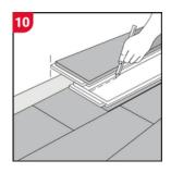
First or last row at uneven walls The first and last rows may need to be trimmed at uneven walls. Scribe the wall line to the plank row as shown, cut and then continue with installation. The last row plank width must be at least 2" wide.
